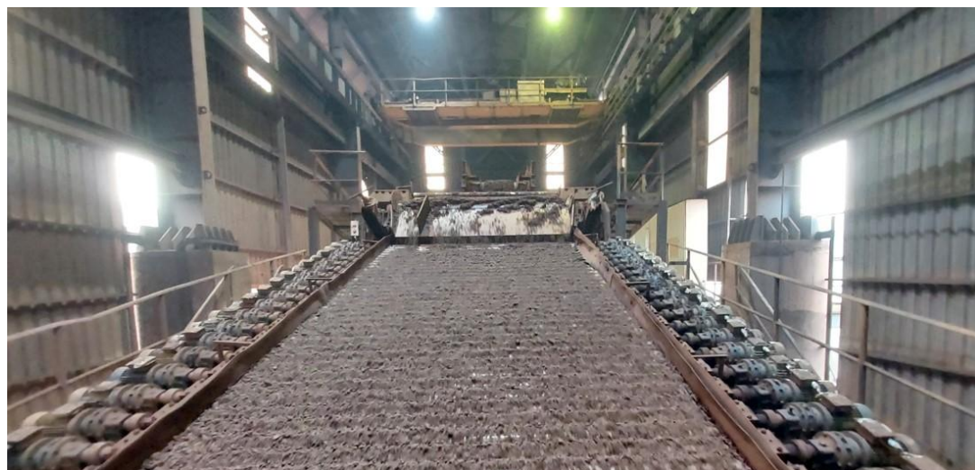
Image 2: Pellet classifier in pellet manufacturing unit
